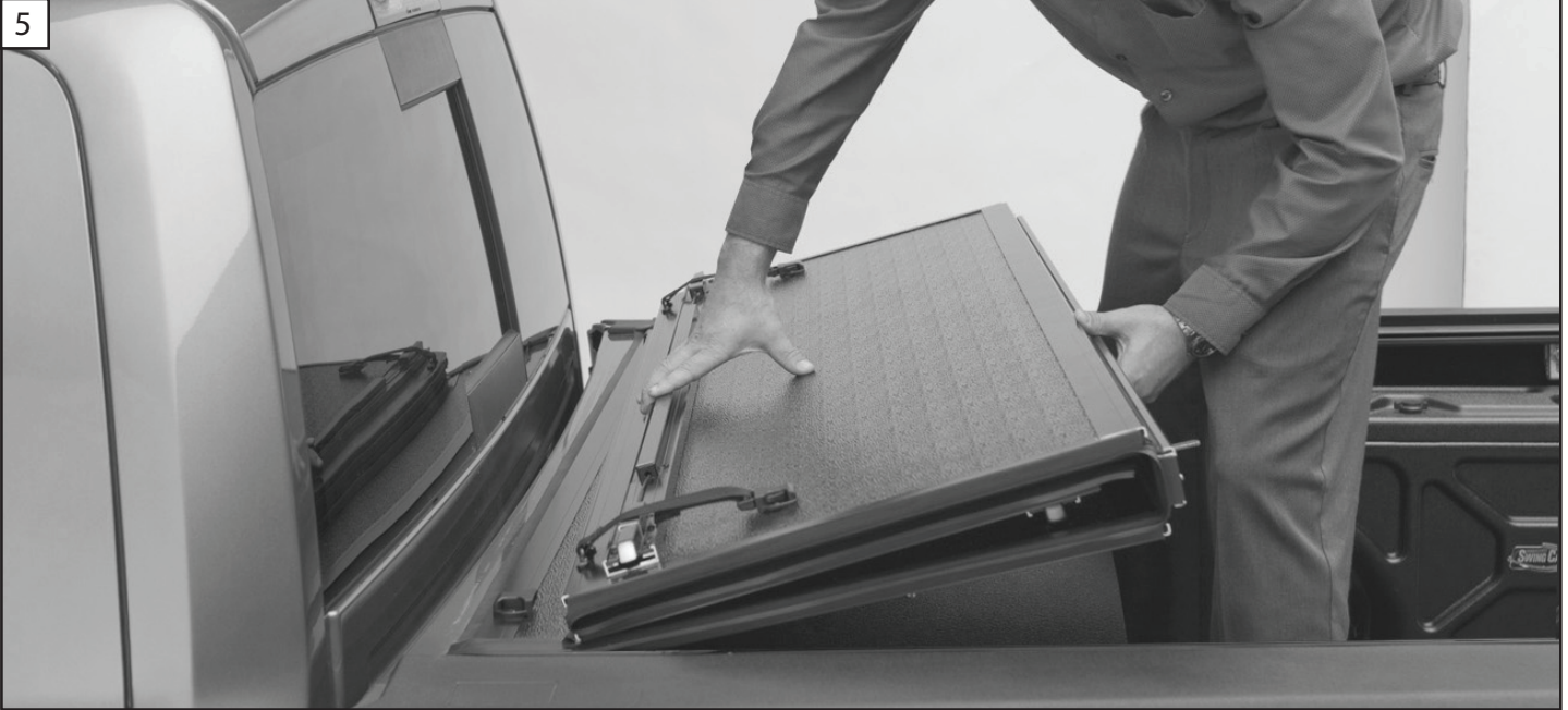
5. Set the tonneau onto the mounting rails, the buckles should be to the front.
